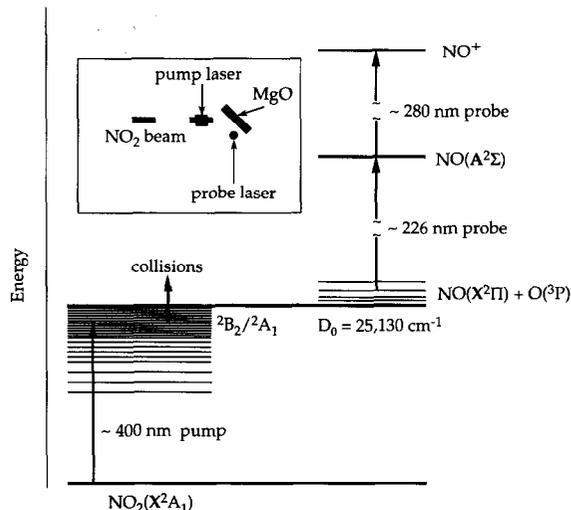
Fig. 1. Schematic energy diagram depicting the CID reaction scheme. Laser excitation prepares internally excited  $\text{NO}_2$  with variable energies below dissociation threshold  $D_0$ . Collision of the excited molecule with the surface leads to its dissociation into  $\text{NO}(X^2\Pi)$  and  $\text{O}(^3P)$ ; the NO product is probed via REMPI. The inset shows the experimental arrangement of the molecular beam, surface, and laser beams.
